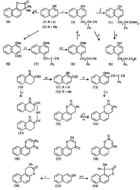
Reagents. i, CH<sub>2</sub>=C(CN)Ph-ZnCl<sub>2</sub>; ii, H<sub>2</sub>O<sub>2</sub>-KOH; iii, KOH- EtOH; iv, pyridine, HCl; v, Zn(CN)<sub>2</sub>-HCl; vi, PhCH<sub>2</sub>·CN-KOH; vii, H<sub>2</sub>/Pd-C; viii, CH<sub>2</sub>=C(Ph)CO<sub>2</sub>Et-AlCl<sub>3</sub>; ix, DDQ- dioxan; x, PhCH<sub>2</sub>·CN-NH<sub>4</sub>OAc.
